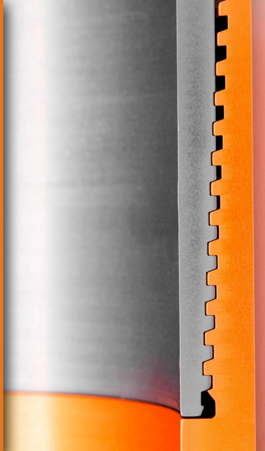
The rugged thread design resists cross-threading and stabbing damage. It also features a reverse load-flank hook thread with a thread compound relief groove.
