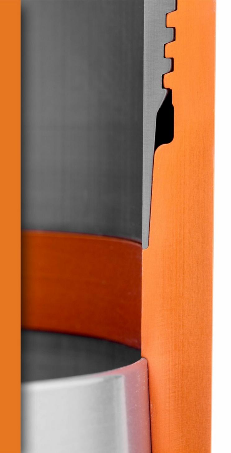
Reverse load-flank hook thread allows for smooth running without galling. This gives EVRlock QB2 greater than 100% pipe body strength in tension. In addition, the steep stabbing flank aids runnability, maintaining greater than 100% pipe body strength in compression.
